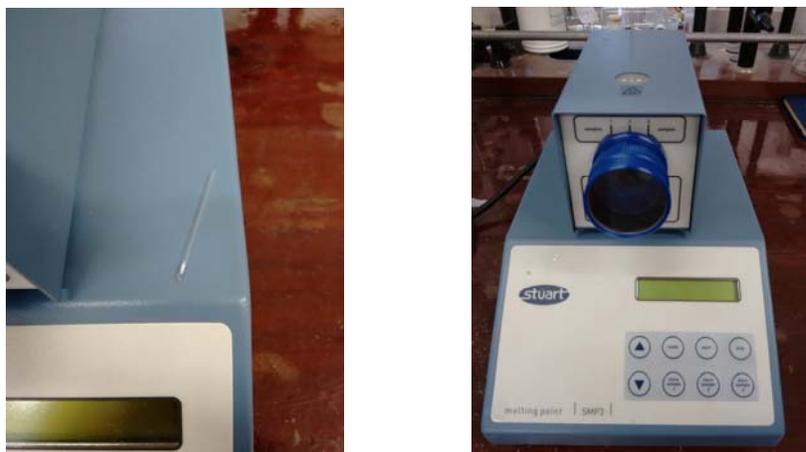
Figure SM 17.8.2 Left - Sample loaded into the sealed capillary; Right- Photo of the apparatus for the determination of the melting point.
