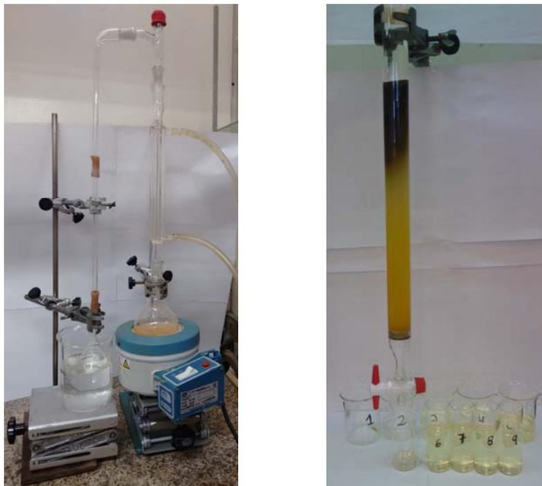
Figure SM 17.8.3 Left - Photo of the apparatus for heating at reflux with a  $\text{H}_2\text{S}$  trap (laboratory session 4); Right- Photo of the apparatus for purification of the product by column chromatography (laboratory session 5).
