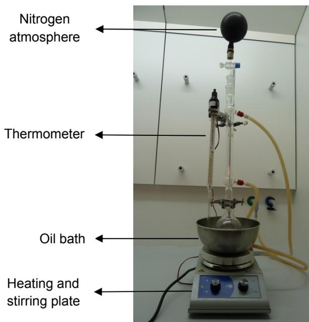
**Figure SM 17.6.2** - Reaction apparatus.
