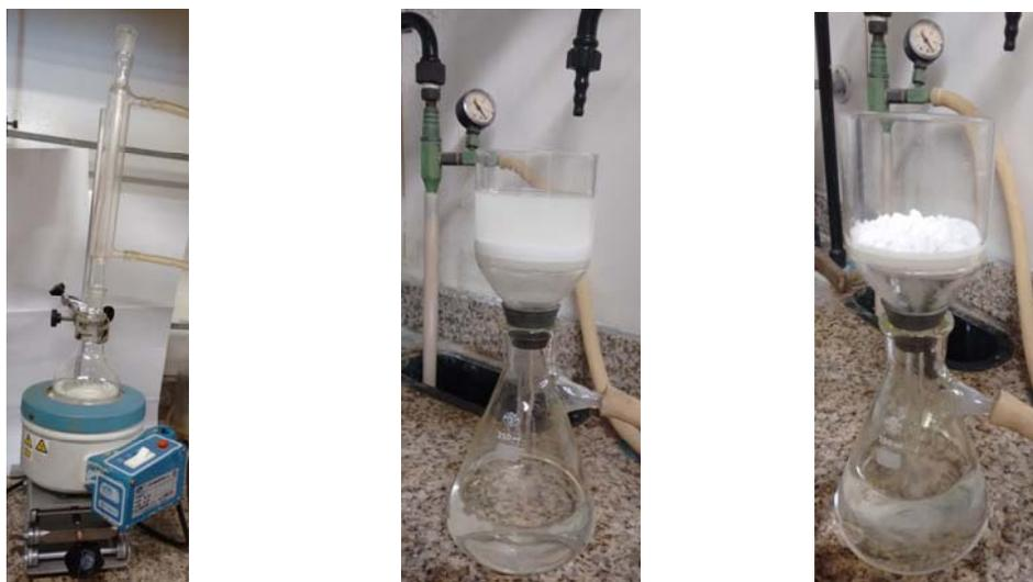
Figure SM 17.8.1 Left - Photo for the apparatus for heating at reflux (recrystallization); centre and right- photos of the vacuum filtration of the recrystallized solid.
