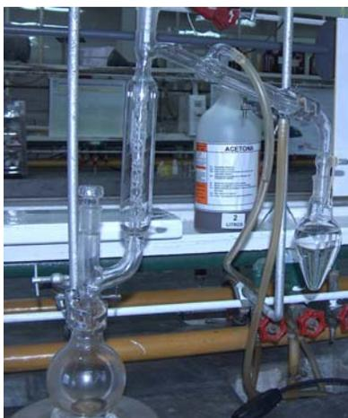
Figure SM 17.4.1 Example of the reaction apparatus for the fractional vacuum distillation.
