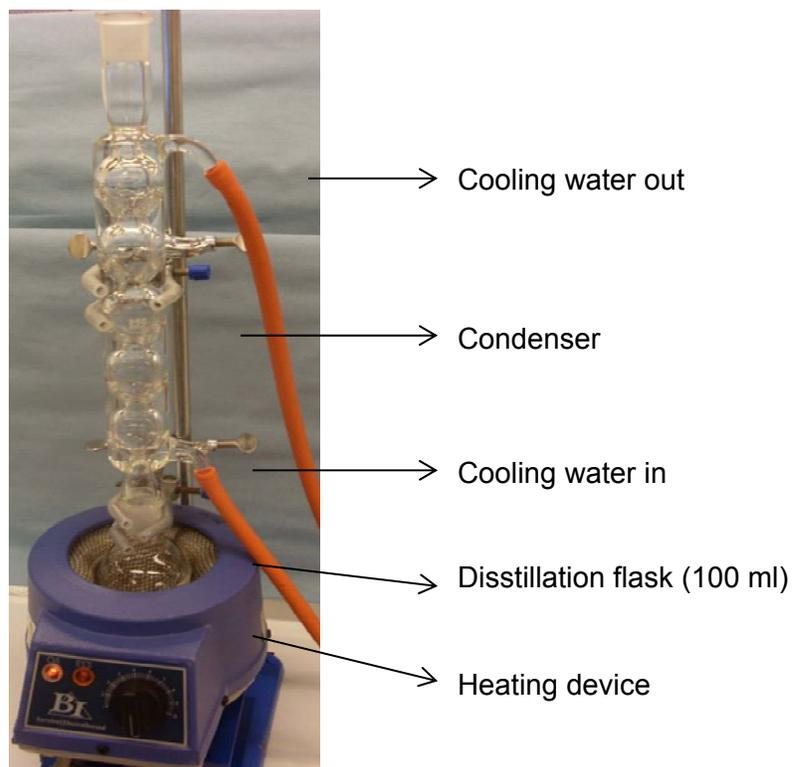
**Figure SM 17.1.1** – The reaction setup. Used to reaction and recrystallizing.
